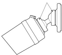
If you have a varifocal lens, remove the cover with the supplied 1/8-inch hollow screwdriver bit. Loosen the focal length and focus locking screws. Adjust according to scene detail. Retighten the screws. Reseat the 0-ring on the cover and reinstall the cover.
